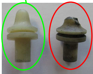
Correct pinball comparing with a worn one
