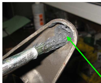
Apply a small quantity of grease
